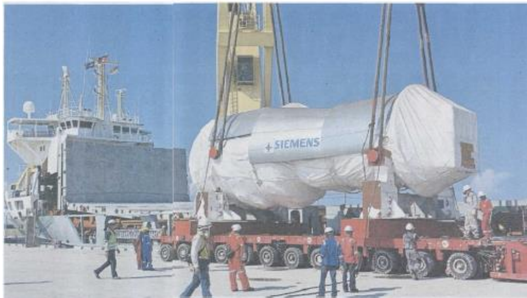
The turbine, which is as heavy as a fully-fuelled A380 Airbus, arrived in Malaysia on the vessel 'MV Annette' on June 6, 2016, and is expected to go online into commercial operation by the middle of 2017.
